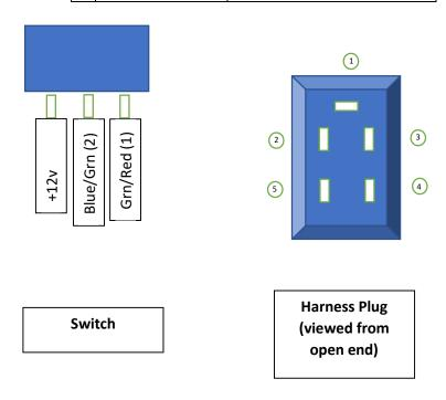
TWO SPEED WIPER MOTOR WIRING LAYOUT
