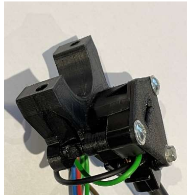
Fig.8. Wiper switch mounted on carrier
