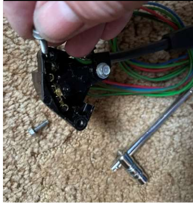
Fig.7. Removing the self-tapping screws.
