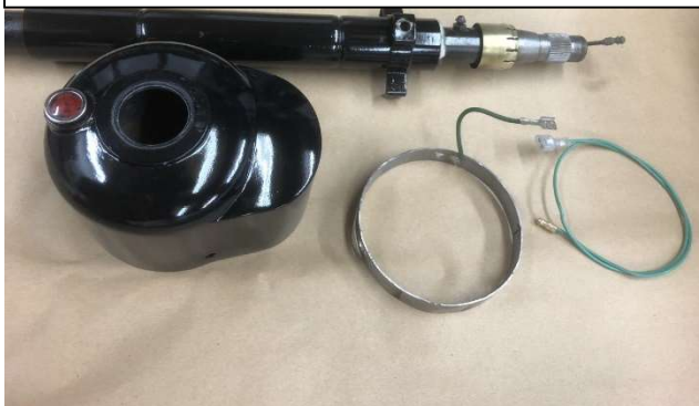
Fig.4 Steering column, new shroud, reinforcing ring (with earth lead) and separate wire for repeater light.
