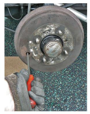
Inspect all pipe unions for leaks, using a good light source, and re-check all nuts for tightness. The bleeding operation will have moved the shoes around a little and they should now be nicely centered so the final job is to adjust the brake (fig. 9). Turn the drum by hand and advance the adjuster until the drum tightens, then back off the adjuster by one click.
