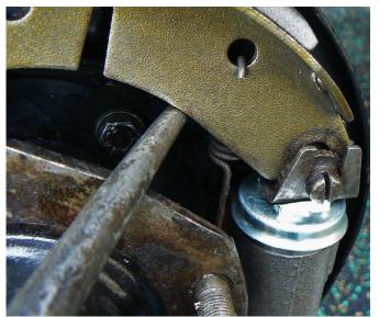
way round, take a photo BEFORE dismantling. Lever the brake shoes up at one end and slip the adjusters out (fig. 3); take off the brake shoes and if in good condition, lay them aside with their springs as found on the car. This will serve as a reminder when reassembling. If the shoes appear worn, damaged or are wet with fluid or oil, replacement will be
