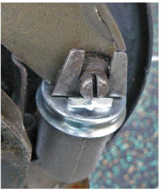
are clean and wound fully back (fig. 7). They must fit snugly into the shallow channel formed on the top of the piston, as in fig. 8.
