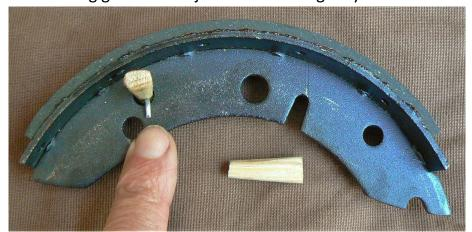
can now go on, as shown, your wooden pegs as seen in fig. 6 will help to keep the spring ends in place. Fit the adjusters last, ensuring that they
