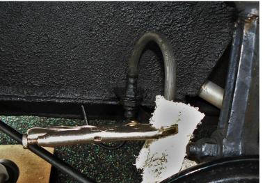
your clean garage floor. Use a pair of grips or a small clamp whilst protecting the hose with rag or cardboard; it doesn't have to be nipped up particularly tightly. This is a good time to inspect the hoses for cracks and replace if necessary.
