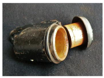
leads quickly to seizure. Fig. 1 shows the rust formed after a short lay-up in damp conditions. Once piston and cylinder have rusted together it is almost impossible to free them without causing damage. If your car is laid up for the winter, it's not a bad idea to give the footbrake a few pumps on a regular basis. It may help to keep the moving
