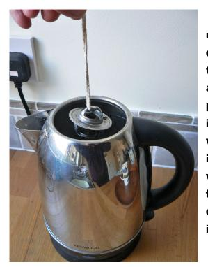
A thermostat may be tested in a rather rudimentary fashion by dangling it in hot water (fig. 5) Boil the kettle and drop the thermostat in. as long as the water is near boiling point the thermostat should open, as in fig. 2. On removing it from the water it should begin to close immediately. If it opens in water which is well below boiling, it is faulty, as is a thermostat which does not begin to close as soon as it is removed from the heat.
