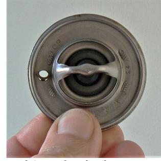
much too early or has been removed, the consequences are less obvious but equally undesirable. The entire amount of coolant is immedately in circulation and the radiator is doing its best to dissipate any heat that comes its way. The engine will boiling will soon occur, generally a very obvious problem which must be dealt with immediately.
