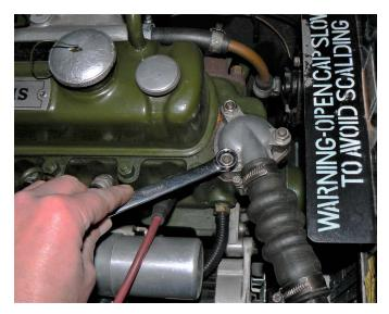
The thermostat is one of the most accessible components of the Minor's engine, see fig. 3; for a general layout of parts see fig. 4. The only preparation needed for removal is to drain the coolant. If the housing has not been taken off for a long time it may well be corroded to its studs, making removal a
