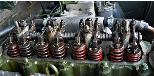
Observe in fig. 3 that two valves are depressed at any one time and the entire set can be checked/adjusted with only two revolutions of the engine.
