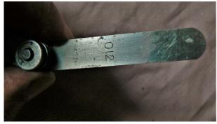
see fig. 2, so make doubly sure you have the right one, .012". If you only have metric feelers, use 0.3mm. Use the starting handle to turn the engine or engage top gear and gently rock the car backwards to set the correct position for adjustment.
