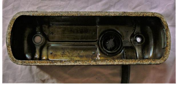
that, as in fig. 7, the fit is perfect. Lay aside for a few minutes to allow for setting during which time the mating face of the cylinder head should be cleaned. There is no need to glue both sides of the gasket; the glue is for positioning, not oil - sealing.
