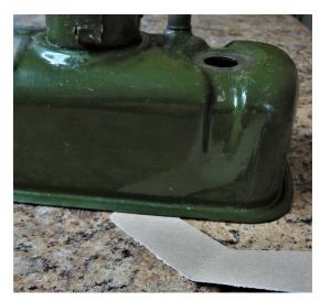
To ensure the best chance of a leak-free result, some care should be taken whilst refitting the rocker cover and its new gasket. First clean the cover scrupulously and examine it for distortion. The sides must be parallel with an even flange all round (fig. 4). Lay the cover on a good flat surface (a worktop is ideal as in fig. 5) and slip a piece of thin card under the edge to test the clearance. Small adjustments can be made by a little
