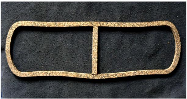
It's hopeless trying to tuck a bendy gasket under the rocker cover and expect it to stay in place whilst you go and find the retaining nuts. A little assistance is required here and by far the best solution is to glue the gasket to the cover.
