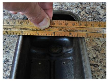
judicious bending; using a hammer will in all probability make things worse! If overtightening has occurred, the area around the securing bolt holes will be distorted and must be brought back to be flat and even to give the sealing rubbers a chance to do their job properly.
