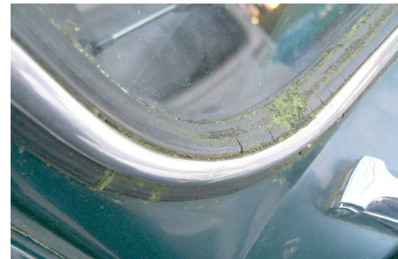
Photo – 1. This screen seal has exceeded its useful life, however, the green fungus is playing its part in sealing the cracks.
