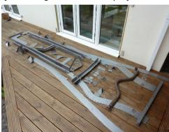
with the option of galvanising—should last a good long time. Work on the 'ex' Dorset Branch Van was progressing nicely at the time of the visit and Brian was poised to fit the new repair piece he had just fabricated, consisting of the front chassis leg sections already joined to the front cross member (under the radiator). Sadly, there was little left of the original ones.
