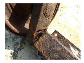
Hello, The trailer started making a strange rumbling noise. On checking I found that the wheel was leaning and the brake drum was rubbing the suspension arm.
