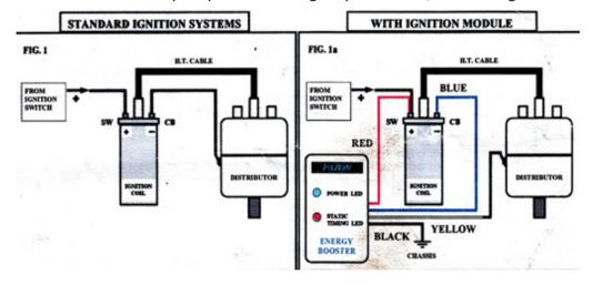
ser in the distributor may be left in place or removed, it makes no difference. Any connectors or extensions to the wiring must be soldered to avoid any problems which could lead to misfiring or a complete breakdown. There is no need to make up any fixing brackets as the 'box' can be wrapped in something to keep it from rattling - I used a piece of innertube - and placed anywhere convenient, as long as it is safe; the one on my car being trapped behind the tie plate
