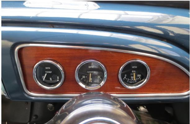
Favourite locations, which will not disfigure your car irreversibly are below the dash on separate brackets or on a panel, usually of wood ( example above ) fitted into the driver's glovebox aperture, thus gaining extra mounting space but preventing its normal use. With a wooden panel you are on your own when it comes to manufacture.
