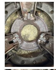
This shows the inner release ring assembly with the three retaining springs fitted but with the top one dislodged on both sides (viewed from inside the clutch)
