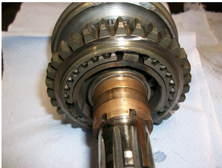
Fig 16—Baulk ring fitted
