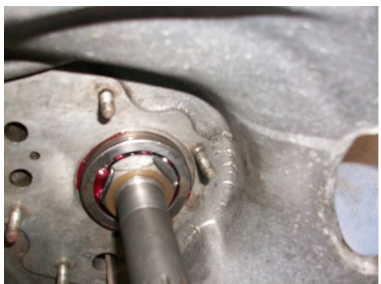
Fig 12—1st motion shaft in with groove visible in bell housing
