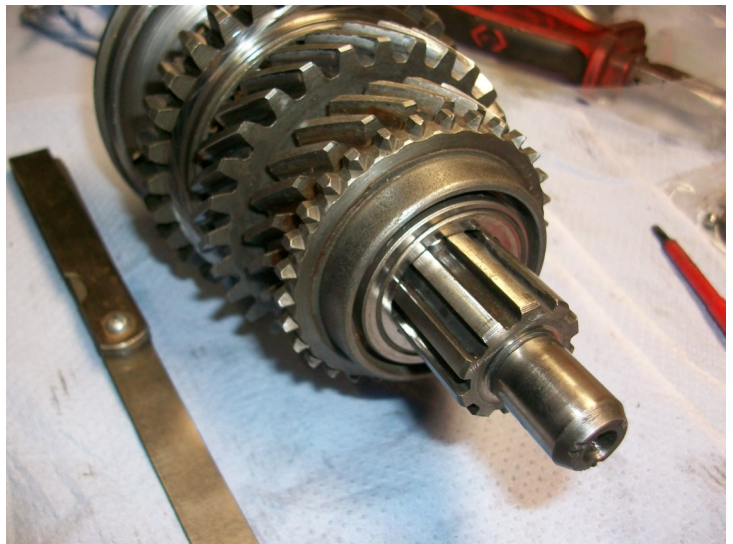
Fig 23—Washer fitted and locked, note pin in splined washer locking it
