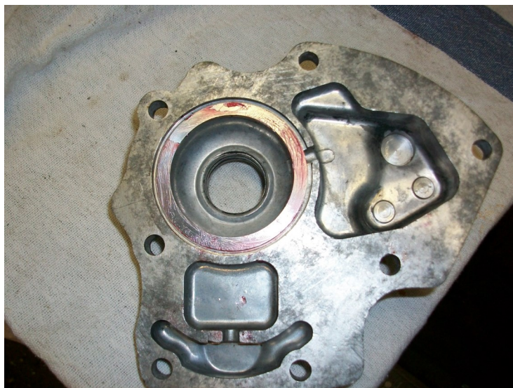
Fig 6—Bearing shims fitted to cover, note the grease
