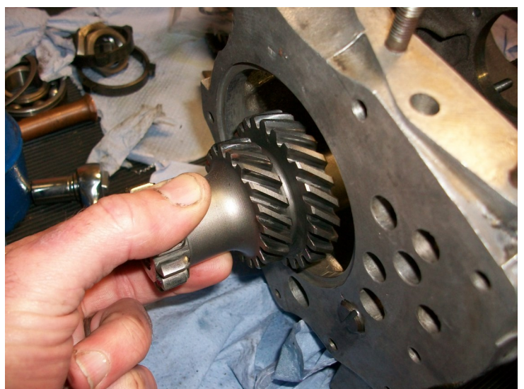
Fig 9—Laygear being fed into the case
