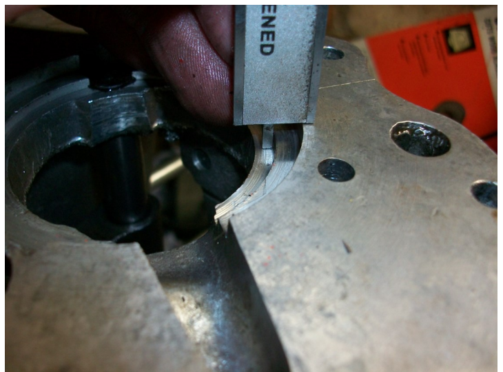
Fig 10—And measure the depth of the recess in the tail housing
