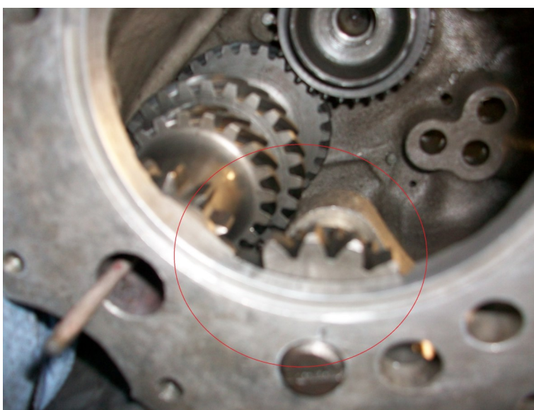
Fig 20—Reverse gear where the cut out must be in the bearing carrier
