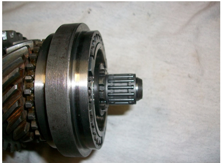
Fig 18—3rd motion shaft nose bearing fitted
