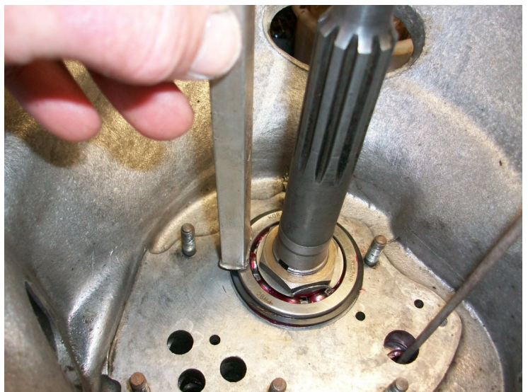
Fig 14—Drifting the bearing to its correct position
