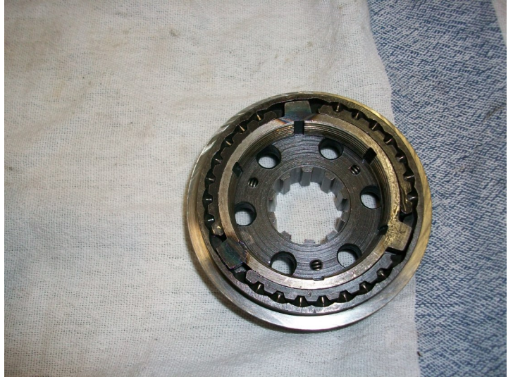
Fig 16—3rd & 4th gear hub, baulk ring fitted, this side is 3rd gear side
