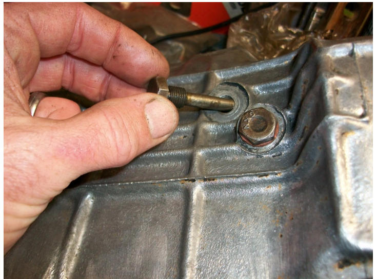
Fig 53—Plain retaining pin goes here
