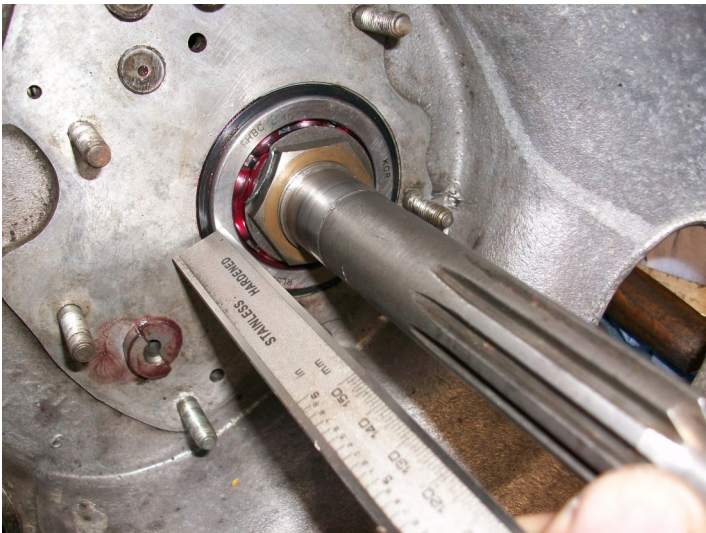
Fig 1—measuring the amount the bearing protrudes
