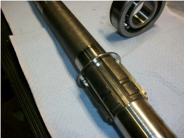
Fig 3—Bearing shim fitted
