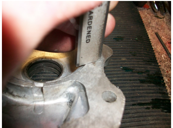
Fig 2—measuring depth of recess in cover
