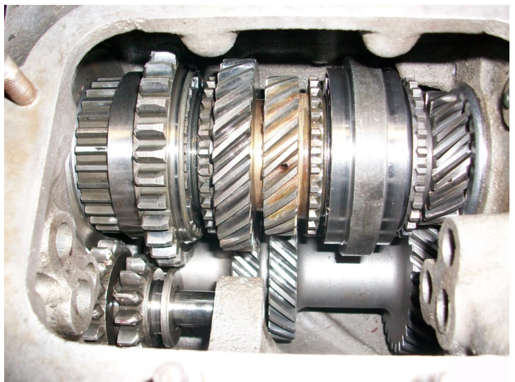
Fig 27—Laygear being brought up into mesh
