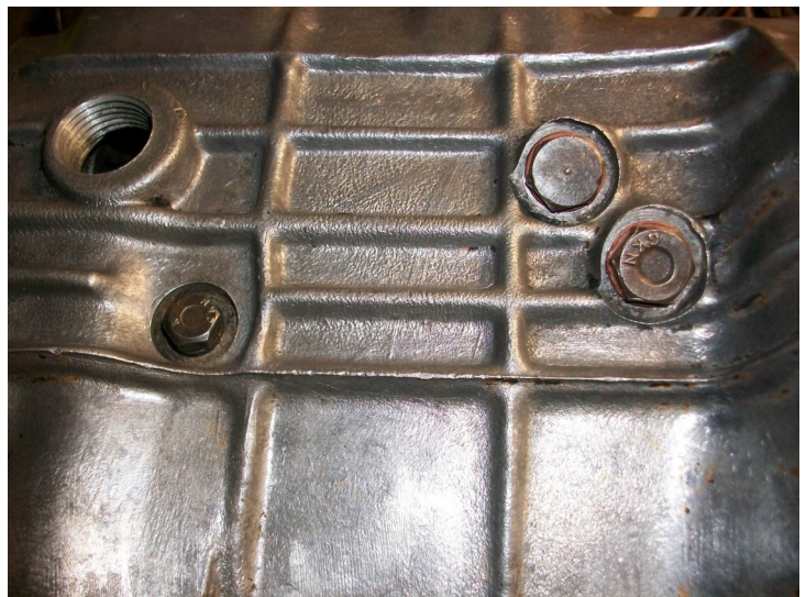
Fig 54—Underside interlock and pin fitted
