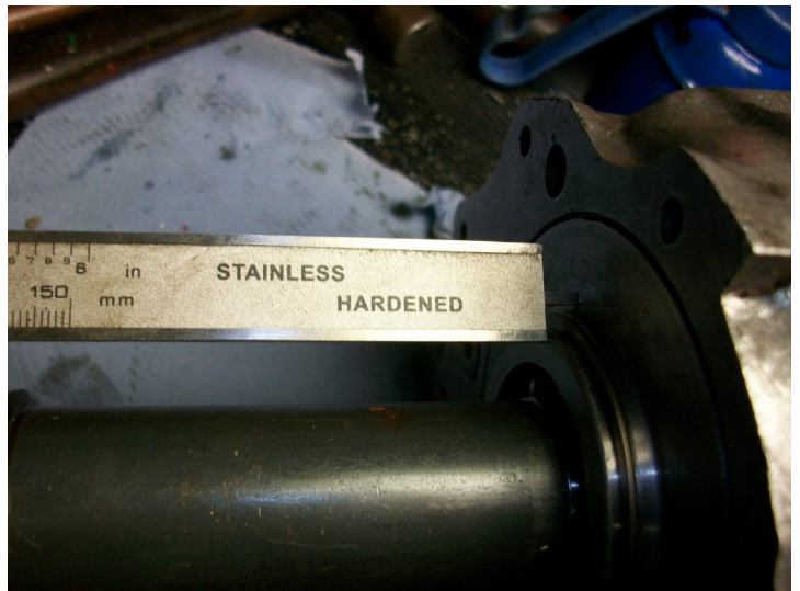
Fig 9—Measure the protrusion of the bearing
