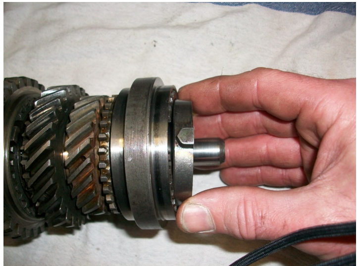
Fig 17—Hub fitted to shaft and baulk ring for 4th gear being fitted
