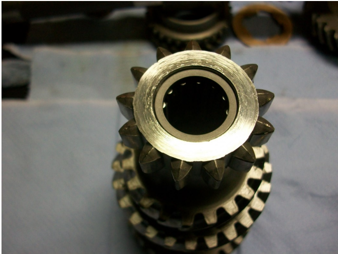
Fig 1—Laygear bearing fitted
