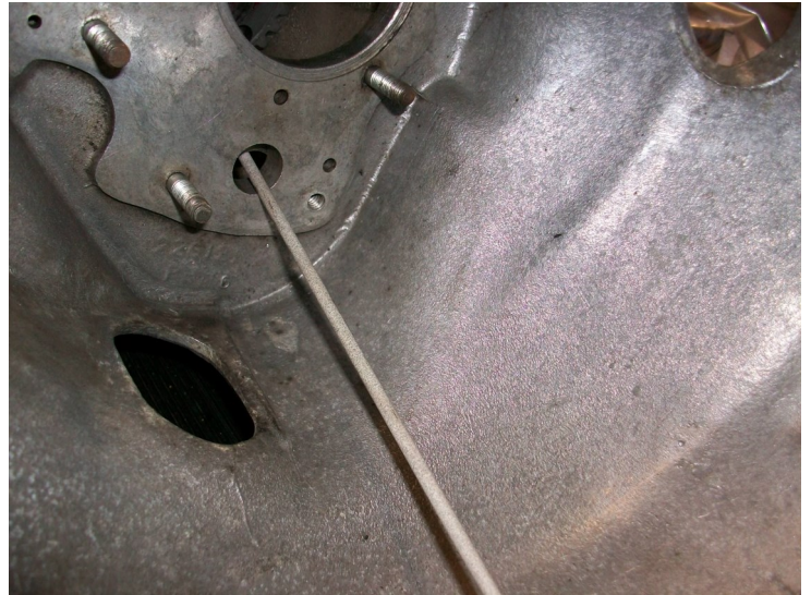
Fig 7—Use of a welding rod to support the laygear
