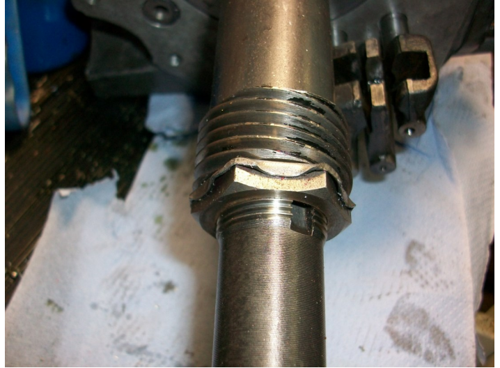
Fig 8—Nut tightened and lock washer bent over
