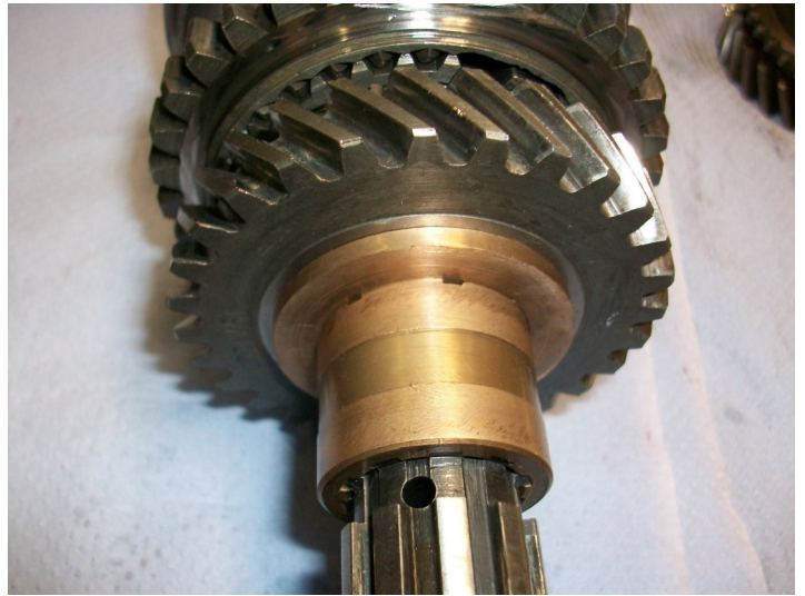
Fig 19—3rd gear bush fitted
