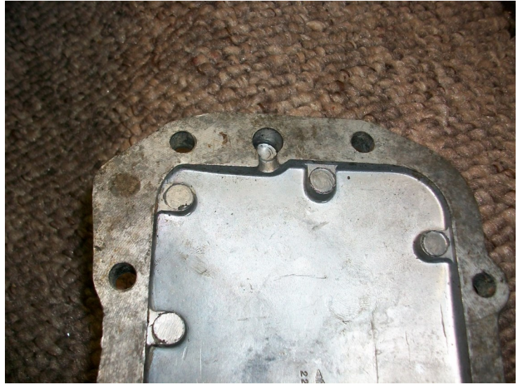
Fig 4—Side cover showing where plunger springs fit
