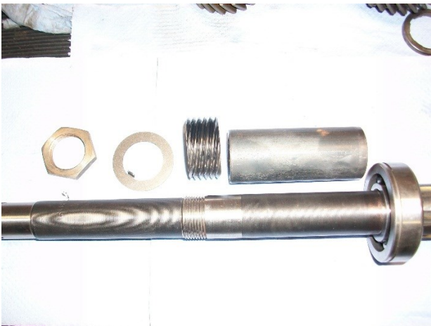
Fig 5—Distance tube, speedo drive, lock washer and nut
