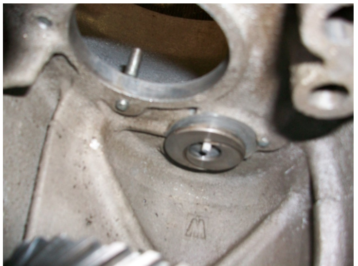
Fig 8—Front thrust washer fitted
