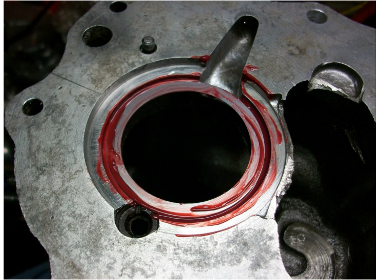
Fig 11—Shim coated with grease and placed in recess
