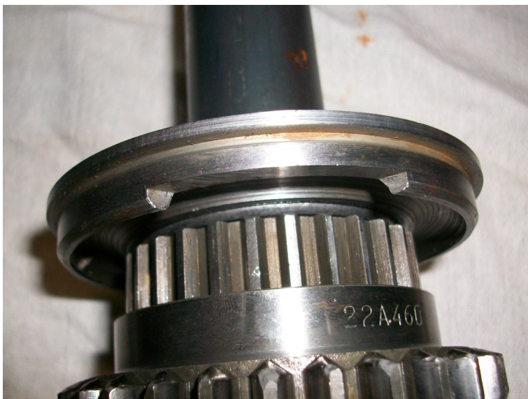
Fig 19—3rd motion shaft bearing carrier showing cut out
