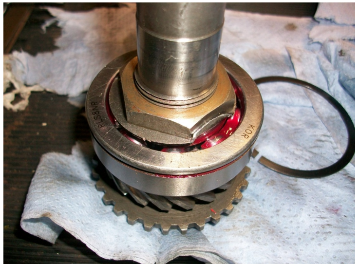
Fig 3—Nut fitted, tightened and washer bent up.
